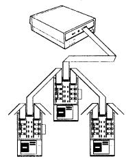
Optionally, the 8 connectors in a multiplexer may each in turn be connected to another multiplexer, called a master multiplexer, forming a two-level network with up to 64 computers. The two-level aspect of such a system is from a hardware viewpoint and doesn't affect the software.
