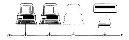
Each computer on the network must have an Omninet interface. The Concept has a built-in Omninet interface. The Omninet interface receives and transmits data at up to 1 million bits per second. Up to 64 devices may share an Omninet network.
